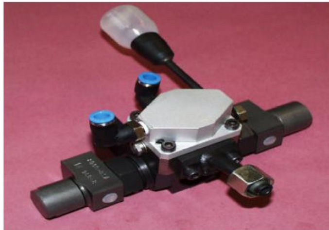
Figure 7: 3-component mixing head for processing expandable graphite and other solids
